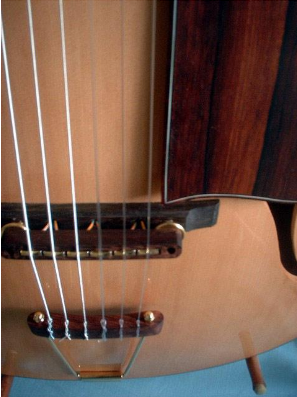
RMC piezo in bridge
